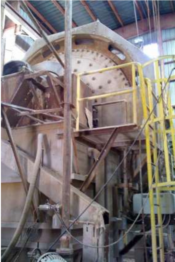
Allis Chalmers 12 x 16 Ball Mill with 1,250 hp motor
