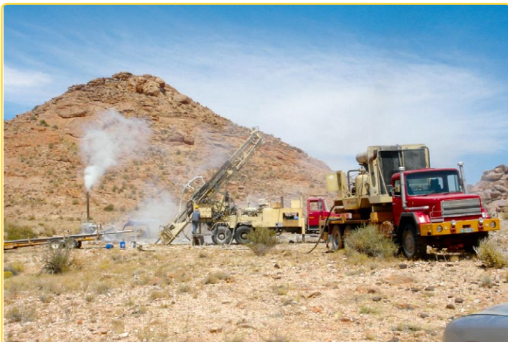
Reverse circulation drilling at Aluriesfontein, October 2008
